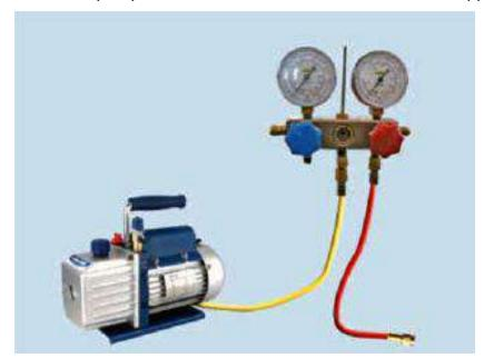
5. When vacuuming the indoor unit and copper pipe, please do not turn on gas / liquid valve, otherwise refrigerant leakage. Vacuum the unit for at least 15 minutes till negative value shown on the pressure gauge, and close the manifold gauge.
