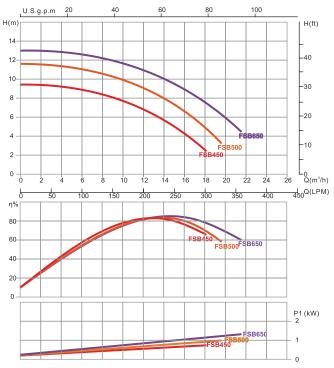
Remarks: Flow curve information based on 220V/50Hz motor.
